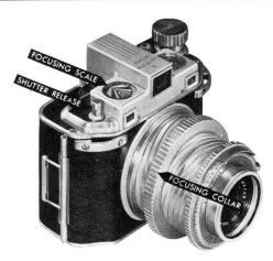
Turn the large FOCUSING COLLAR on the lens barrel to bring the lens to picture-taking position. As the lens is brought forward, the FOCUSING SCALE on the top of the camera automatically revolves to indicate the distance for which the camera is focused.
